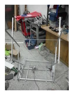
(In order to rise to the height of nearly two meters the basket, we use cross-agency to meet our needs. To increase the stability of its institutions in each node using an aluminum throughout, making it a high stability of the lifting platform.)
