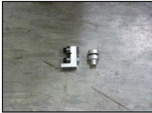
左為軸承滾輪式、右為滑槽輪 Left bearing roller type, right chute wheel
